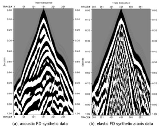
Figure 4: Calculated shot gather with acoustic and elastic modeling method.
