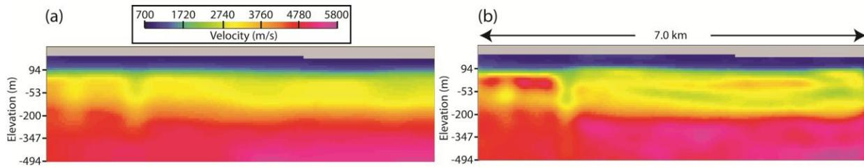
Figure 8. Comparison of cross sections between the traveltome tomography model (a) and the waveform tomography model (b).
