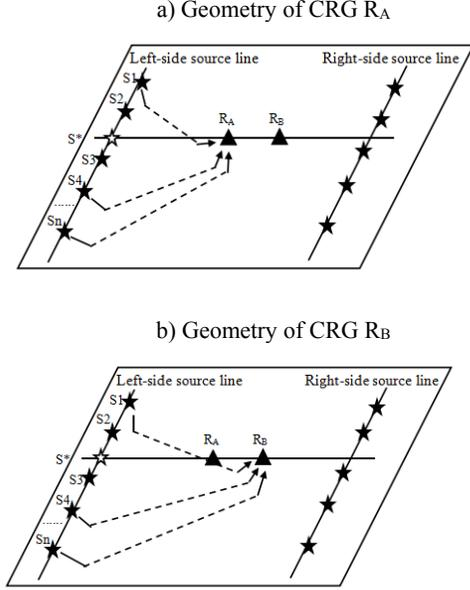
Figure 2: Geometry of sources and receivers. One left-side source line and one right-side source line for the receiver pair are shown. a) Geometry of a common receiver gather for receiver  $R_A$  and the integrated source line. b) Geometry of a common receiver gather for  $R_B$  and the integrated source line. The hollow star represents one of the stationary sources for the chosen receiver pair.
