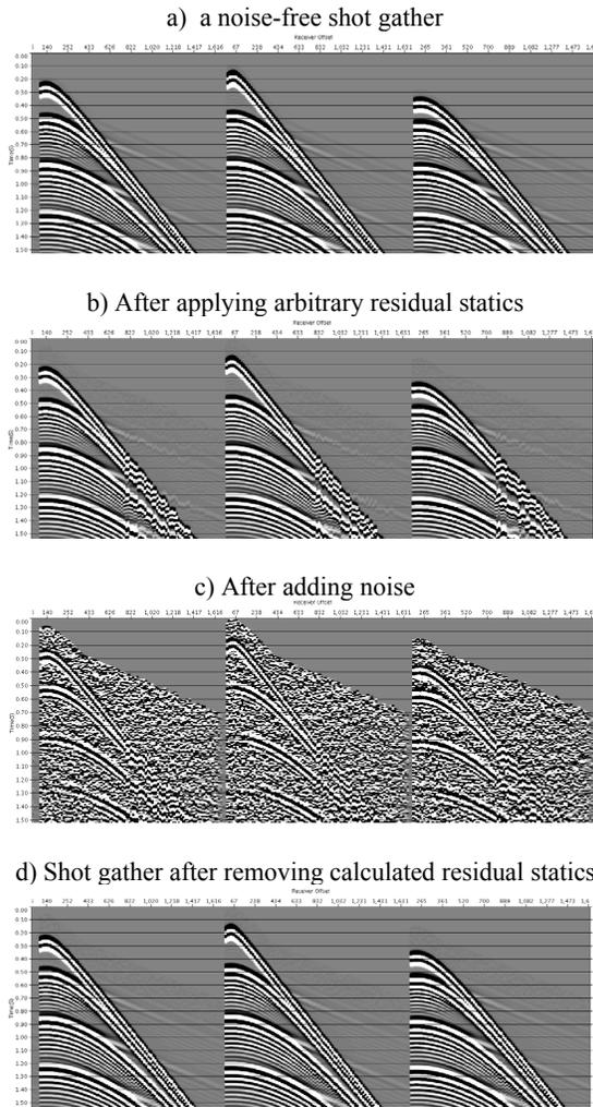
Figure 4: a) A noise-free shot gather b) Apply arbitrary statics between -20 ms and 20 ms to the shot gather c) Add random noise with signal-to-noise ratio of 2 to the shot gather d) The shot gather after removing calculated residual statics
