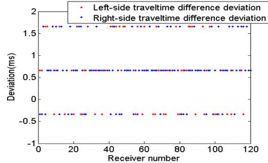
Figure 5: Traveltime difference deviation from stationary traveltime difference for each receiver pair after applying 3D SVI.
