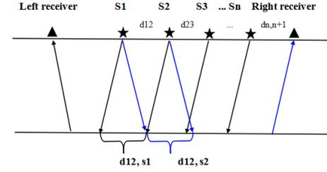
Figure 3: a) Sketch for receiver pair obtaining the signal from both left and right sources, black line represents the refraction raypath from the left source and blue line denotes the signal from the right source. b) Sketch for source pair generating the signal to both left and right receiver, black line represents the refraction raypath to the left receiver and blue line denotes the signal to the right receiver.
