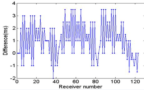
Figure 7: Difference of true residual statics and calculated residual statics.
