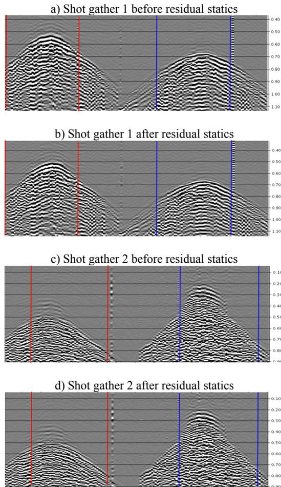
Figure 8: a) Shot gather 1 before residual statics. b) Shot gather 1 after applying residual statics. c) Shot gather 2 before residual statics. d) Shot gather 2 after applying residual statics. The traces between two red/blue lines are received by receivers after applying residual statics.
