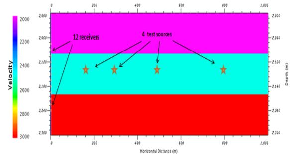
Figure 1: Velocity model and acquisition geometry with four test sources and 12 receivers in the well.
