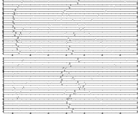
Figure 6: Synthetic waveforms for the first test source with the distance of 150 m. (a) Top panel: horizontal component waveforms for 12 receivers; (b) Bottom panel: vertical component waveforms.
