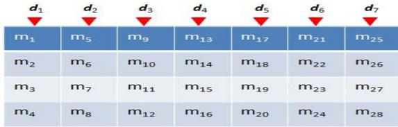
Figure 1: A 2D model structure. From  $m_1$  to  $m_{28}$  are model parameters to be inverted. From  $d_1$  to  $d_7$  are data measured on the surface. Red triangles are receivers on the surface.
