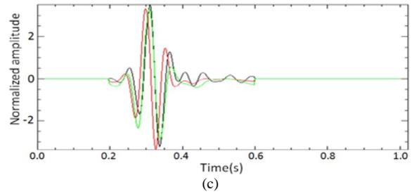
Figure 7: Waveform comparison. Black line represents true data, red line is for initial model and green line is for inversion result after 10 iterations. (a) The 4<sup>th</sup> traces comparison. (b) The 17<sup>th</sup> traces comparison. (c) The 20<sup>th</sup> traces comparison.
