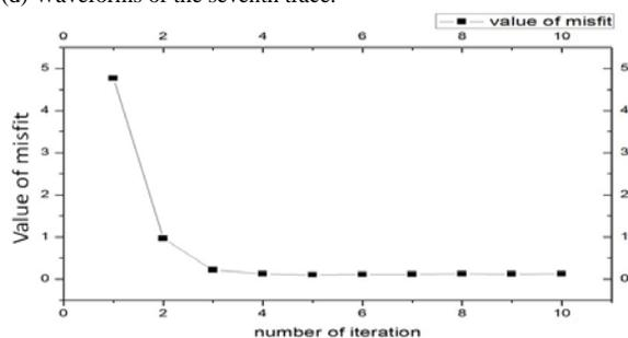
Figure 4: Inversion data misfit of waveforms versus iteration number.
