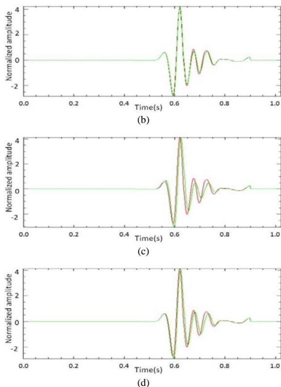
Figure 3: Waveform comparison of the inversion. Black line is for true model, red line is for initial model and green line is for inversion result after 10 iterations. (a) Waveforms of the first trace. (b) Waveforms of the third trace. (c) Waveforms of the fifth trace. (d) Waveforms of the seventh trace.
