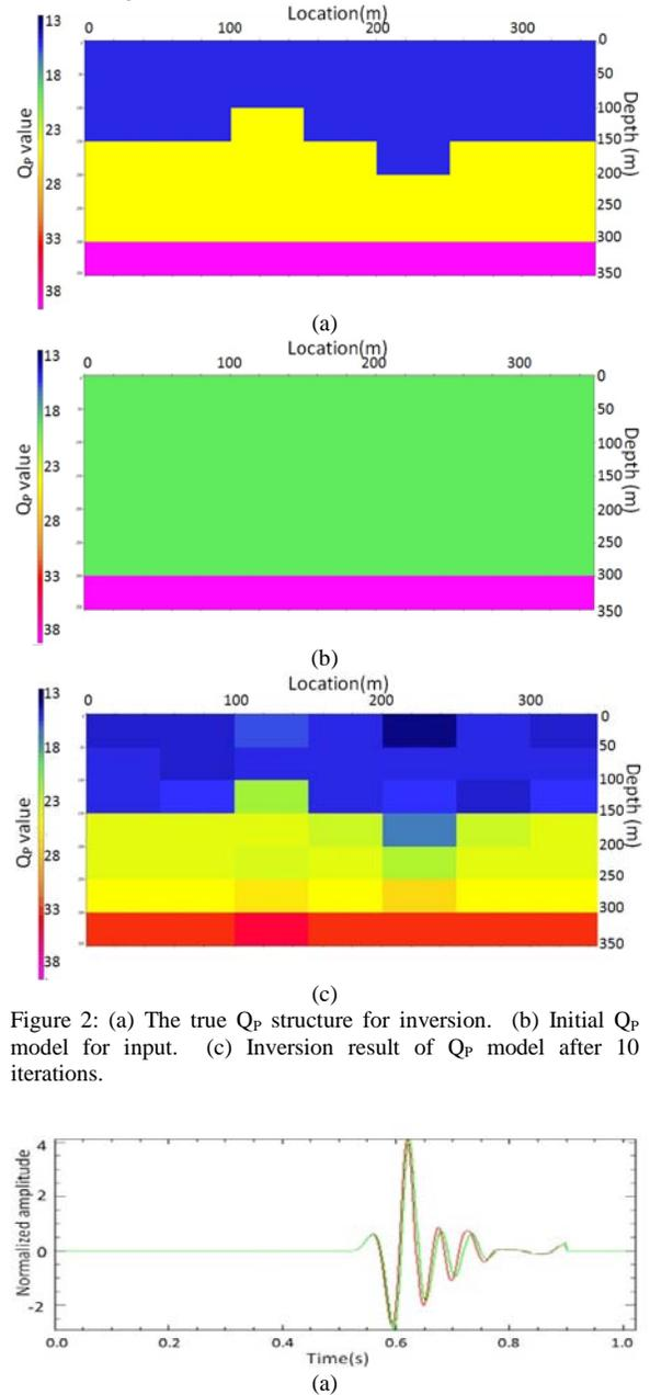
Figure 2: (a) The true  $Q_p$  structure for inversion. (b) Initial  $Q_p$  model for input. (c) Inversion result of  $Q_p$  model after 10 iterations.
