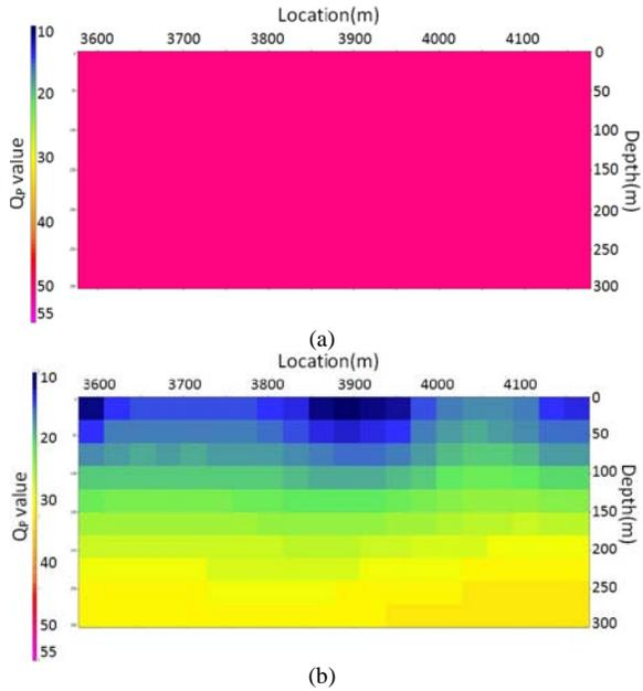
Figure 6: (a) The initial  $Q_p$  structure. (b) Inversion result of  $Q_p$  model after 10 iterations.
