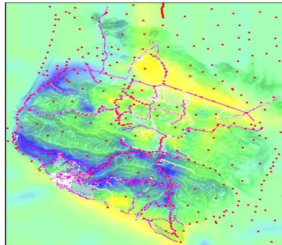
Figure 1: Geometry of seismic acquisition (source in magenta and receiver in white) and gravity observation (red dots).
