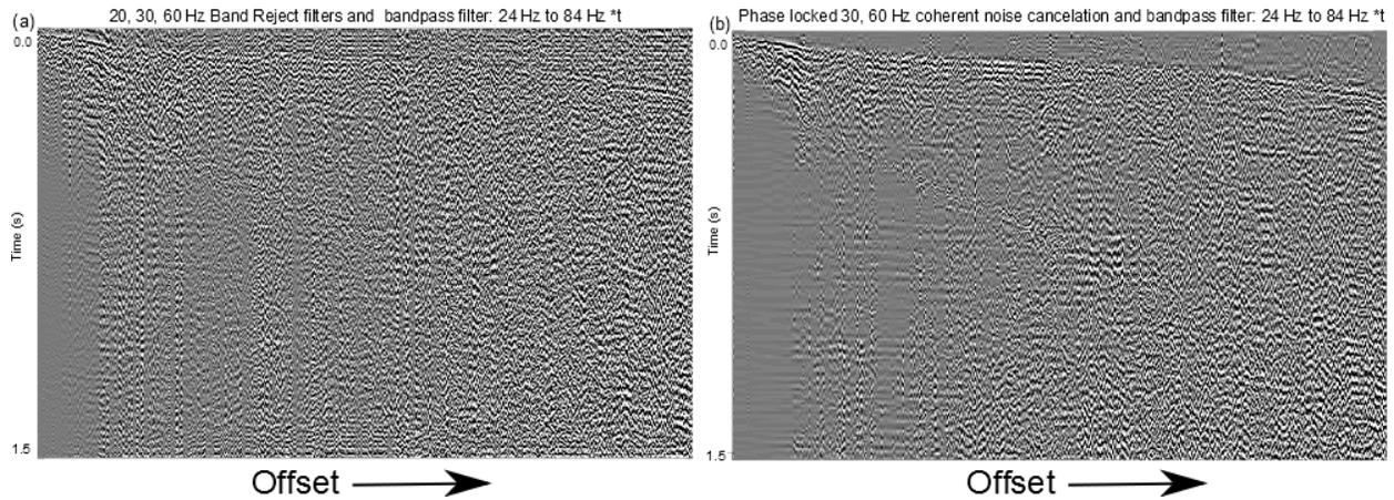
Figure 3: Shot gather with bandpass filter from 24 Hz to 84 Hz from within the power plant area. Bandrejection filters at 20 Hz, 30Hz, and 60 Hz are also applied in (a). Phase-locked coherent noise cancellation is used in (b). Traces are ordered by offset from left (~10 m) to right (~600 m).
