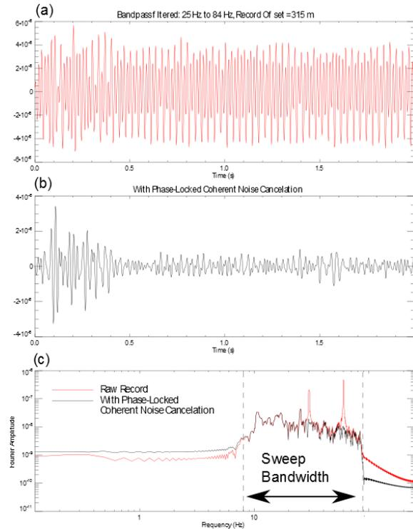
Figure 2: Bandpass-filtered trace (a), phase-locked noise attenuation result (b), and Fourier amplitude (c) of (a) and (b).
