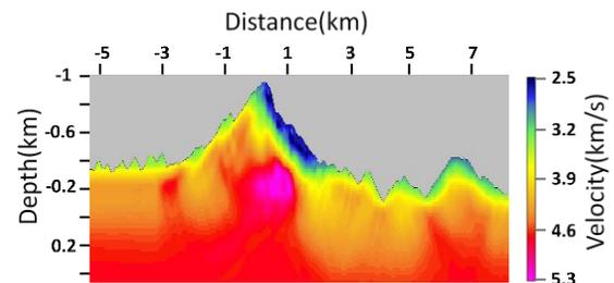
Figure 3: Sichuan data experiment: a) Initial velocity model; b) Traveltimes tomography solution; c) Waveform inversion solution; d) Joint traveltimes and waveform inversion solution.
